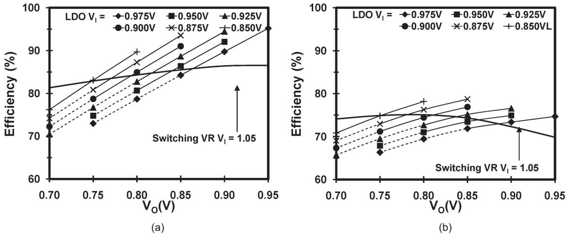
Fig. 5. Efficiency comparison between switching and LDO VRs. The efficiency of (a) the on-chip (the second stage) only and (b) both the off- and on-chip (the first and second stages) are considered.
