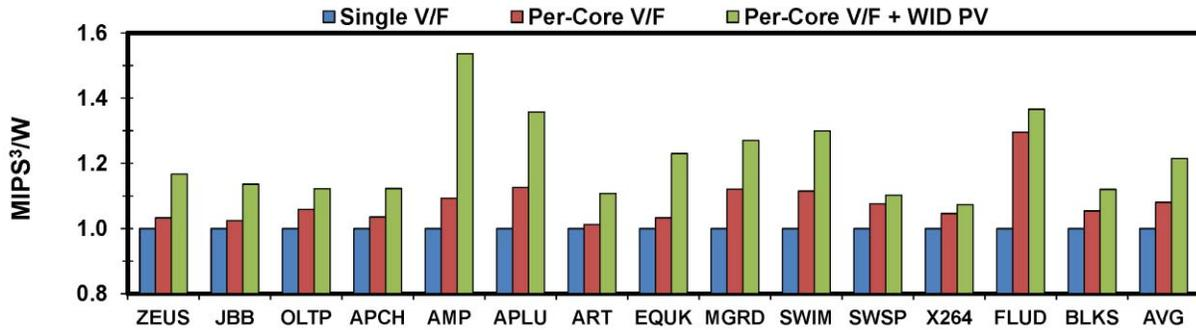
Fig. 1. MIPS<sup>3</sup>/W comparison of eight-core processors supported by a single V/F domain, per-core V/F domains, and per-core V/F domains exploiting WID PV. Each DVFS interval is composed of 10 million instructions.
