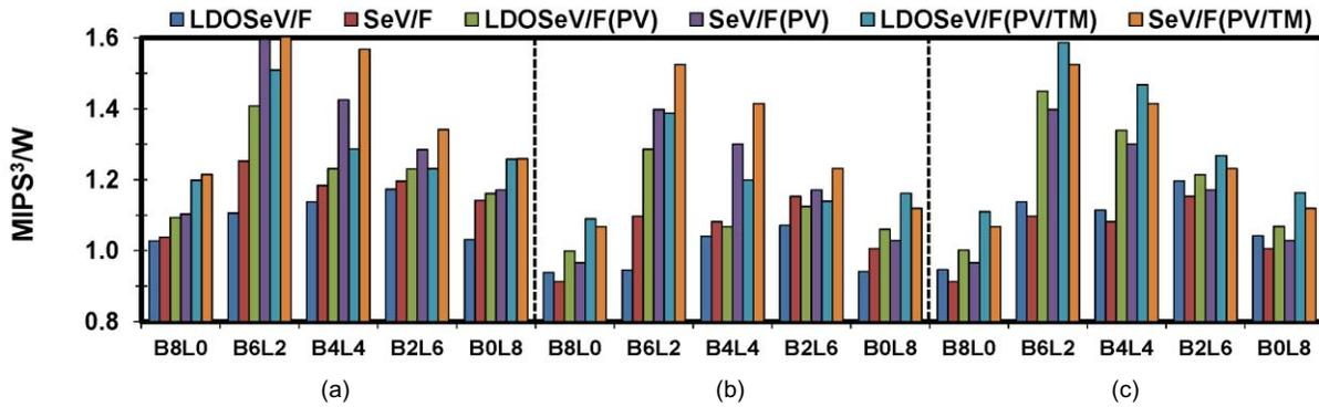
Fig. 8. MIPS<sup>3</sup>/W comparison of eight-core processors supported by LDO (algorithms beginning with the LDOSeV/F prefix) and switching VRs (algorithms beginning with SeV/F). The power loss by on- and off-chip VRs (a) is not included and (b) is included. The  $V_I-V_O$  constraint is removed for LDO VRs in (c) while the power loss by on- and off-chip VRs is accounted for.
