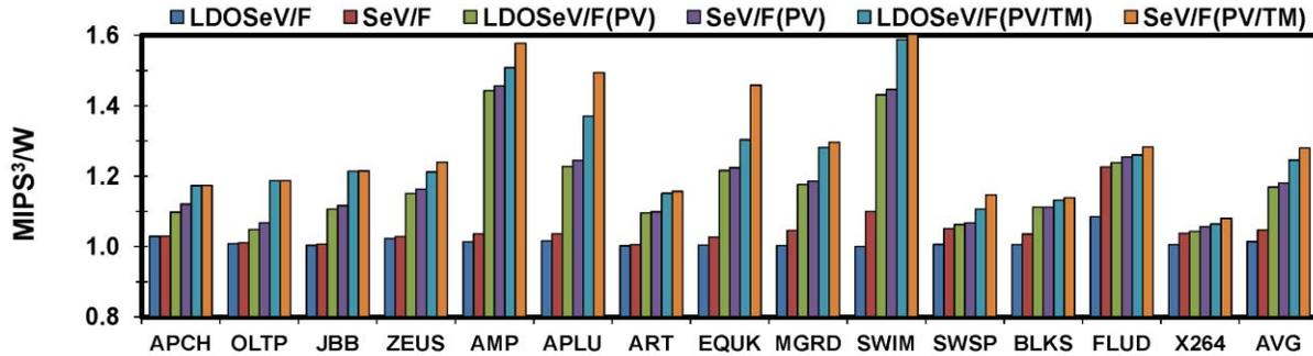
Fig. 6. MIPS<sup>3</sup>/W comparison of eight-core processors supported by LDO (algorithms beginning with the LDOSeV/F prefix) and switching VRs (algorithms beginning with SeV/F). All results are normalized to a processor with ShV/F and *do not* include the power loss by both the on- and off-chip VRs. Each interval is comprised of ten million executed instructions.
