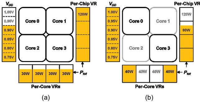
Fig. 2. Impact of splitting the chip-wide voltage domain into per-core voltage domains on the overall VR capacity. (a) All cores are active and consume a total of 120 W. (b) Only two cores are active.
