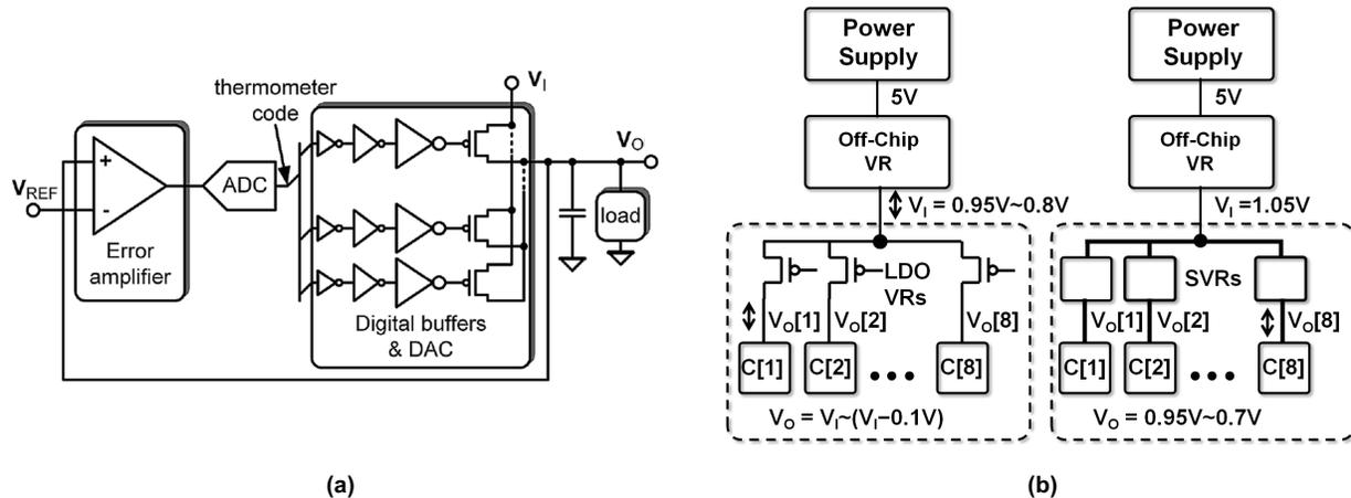
Fig. 4. (a) A typical LDO VR architecture; the image is reproduced from [18]. (b) An example of  $V_I$  and  $V_O$  ranges of LDO VRs in the left and switching VRs denoted by SVRs in the right for supporting per-core voltage domains; for illustration purposes, we ignore the default voltage drop of the LDO VRs due to the small resistance of the fully turned-on PCPG devices in the figure. “C[i]” in (b) denotes core  $i$ .
