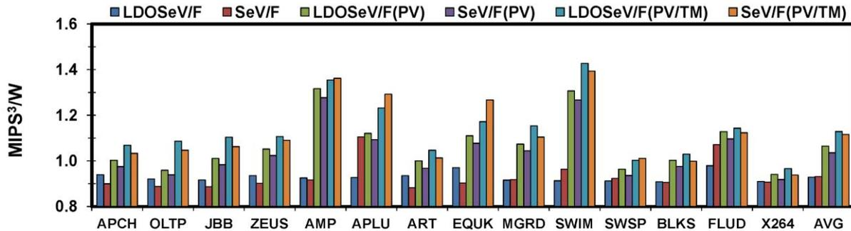
Fig. 7. MIPS<sup>3</sup>/W comparison of eight-core processors supported by LDO (algorithms beginning with the LDOSeV/F prefix) and switching VRs (algorithms beginning with SeV/F) including the power loss by both on- and off-chip VRs. All results are normalized to a processor with ShV/F and include the power loss by the off-chip VR. Each interval is composed of ten million executed instructions.
