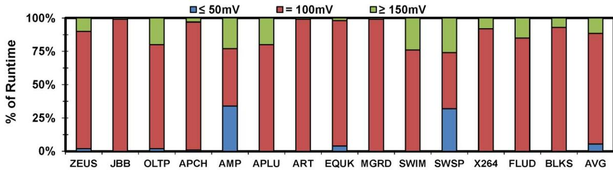
Fig. 3. Fraction of execution intervals exhibiting equal to or less than 50 mV, equal to 100 mV, and equal to or larger than 150-mV voltage differences between cores for the “Per-Core V/F” case presented in Fig. 1.
