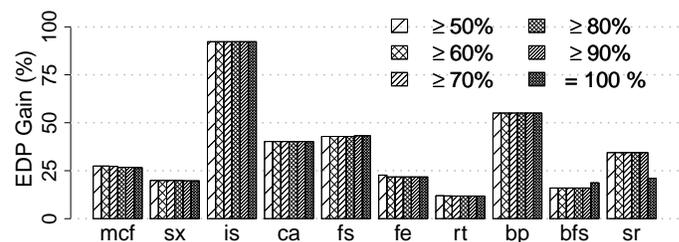
Fig. 9: EDP gain under **recalculation+prediction** as a function of value locality threshold for prediction.
