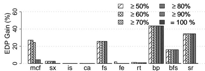
Fig. 8: EDP gain under **prediction** as a function of value locality threshold for prediction.
