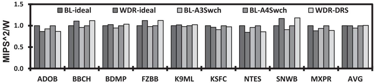
Figure 3: Energy efficiency of big.LITTLE (BL) versus WDR. BL-ideal, BL-A3Swch, and BL-A4Swch correspond to big.LITTLE with no switching overhead, switching overhead modeled after AMBA3, and AMBA4, respectively. WDR-ideal, and WDR-DRS ignore the power overhead incurred by a practical WDR implementation.
