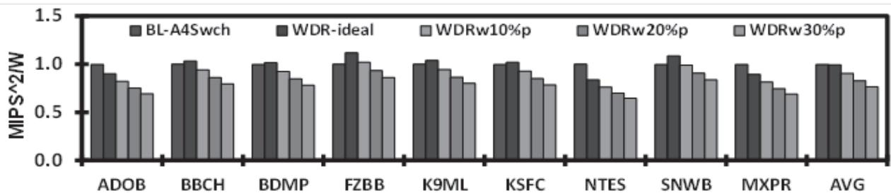
Figure 7: Sensitivity of  $MIPS^2/W$  to the power overhead of WDR of 10%, 20% and 30%.
