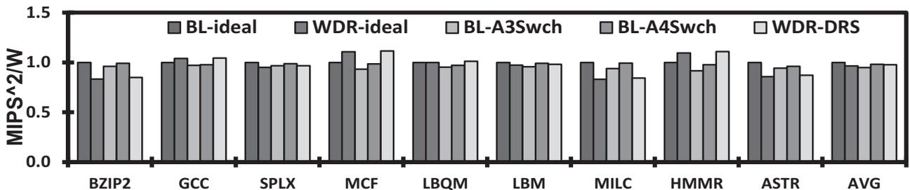
Figure 6:  $MIPS^2/W$  comparison of big.LITTLE (BL) architecture and WDR for single-threaded applications.
