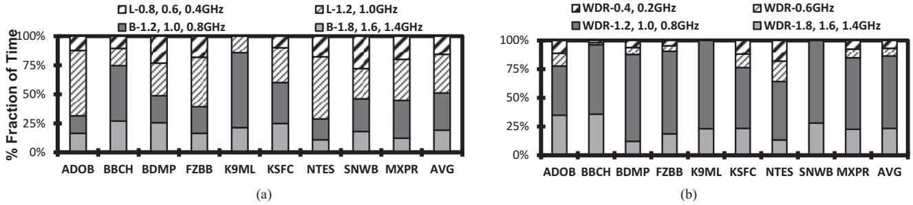
Figure 4: Fraction of time spent in different V/F states of big.LITTLE (a) and WDR (b) architectures, to achieve the energy efficiency reported in Figure 3. The shaded boxes show the % time spent in LITTLE cores for big.LITTLE, and in NTV for WDR, respectively.
