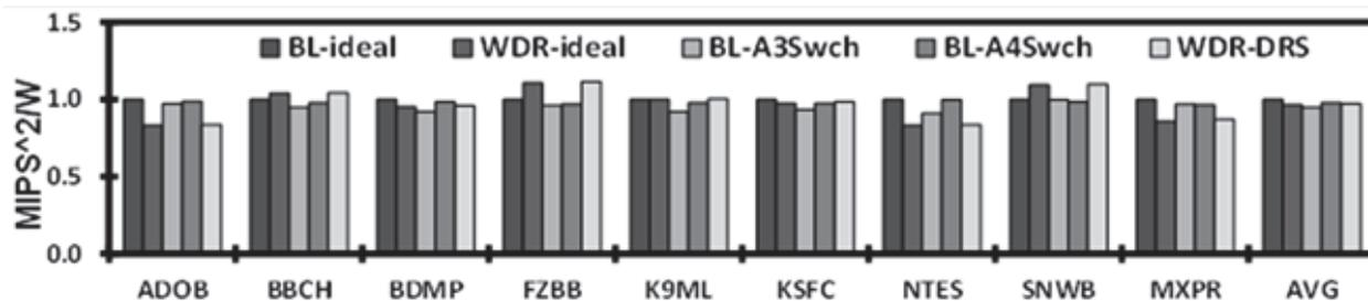
Figure 8:  $MIPS^2/W$  comparison of big.LITTLE (BL) supporting CPU migration and WDR supporting per-core voltage domains
