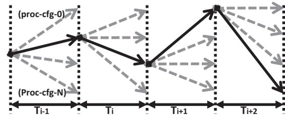
Figure 2: Oracular greedy optimization to find the most energy-efficient processor configuration per interval in big.LITTLE, WDR, and WDR-DRS architecture.
