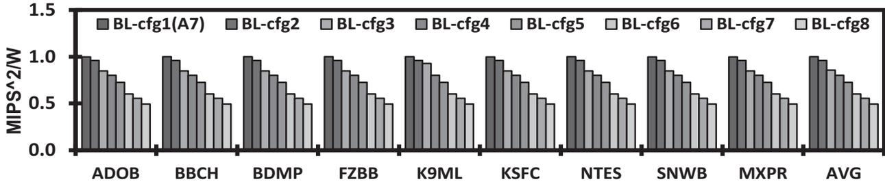
Figure 5:  $MIPS^2/W$  of BL implemented using a pair of cortex-A15 as the big core, and different versions of cortex-A7 as the LITTLE core.
