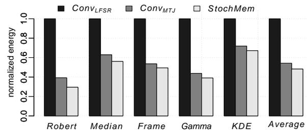
Fig. 5: Energy consumption normalized to  $Conv_{LFSR}$ .
