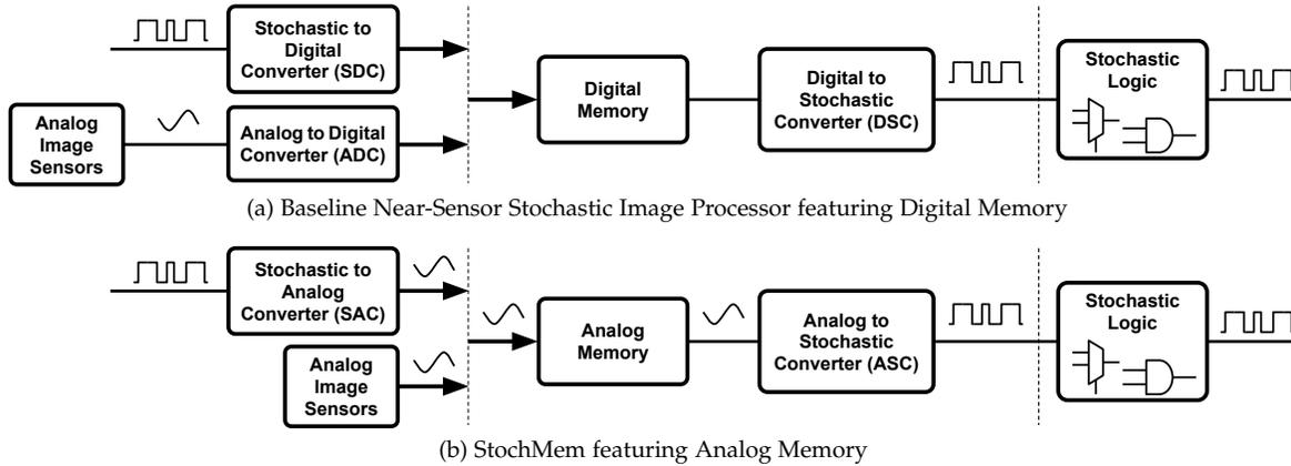
Fig. 1: Baseline Near-Sensor Stochastic Image Processor vs. StochMem.
